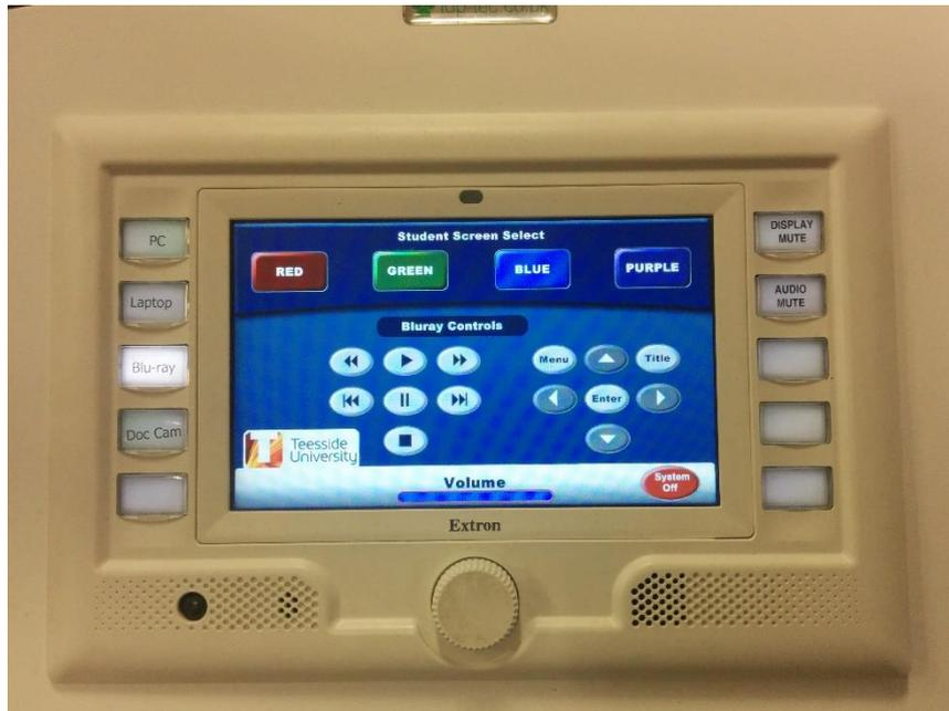
Figure 2 - Control panel showing Blu-ray controls
